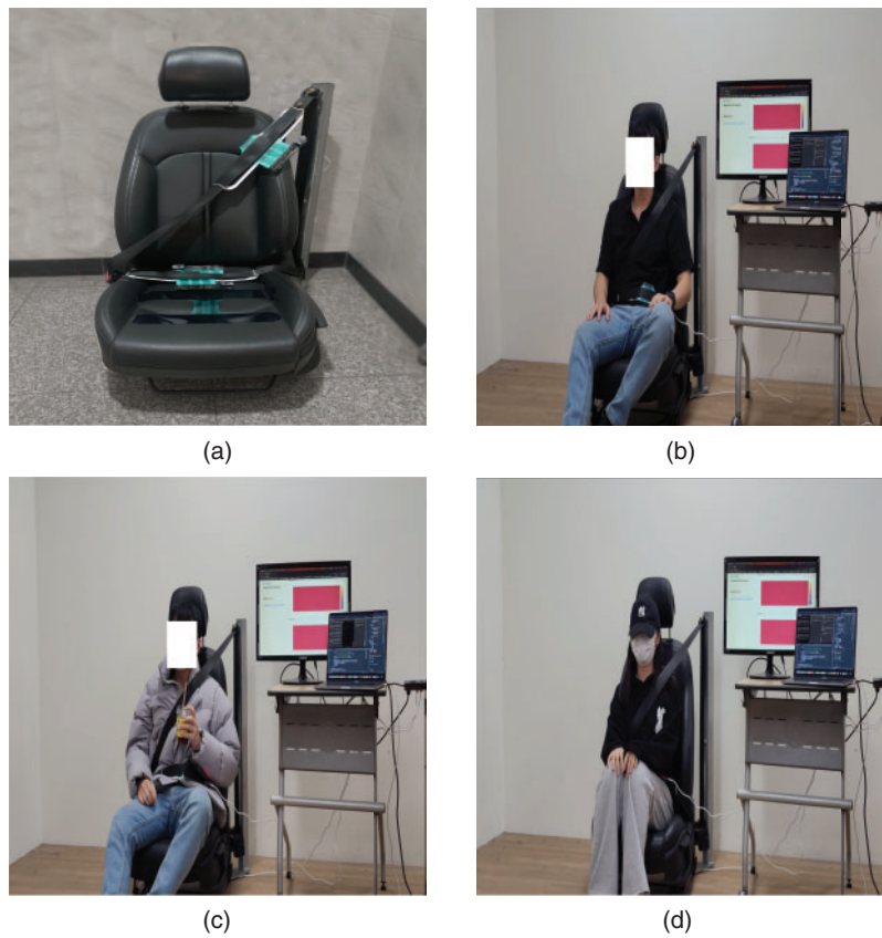
Figure 3: Illustrations show the testbed of data collection experiments: (a) Driver seat attached with belt and seat pressure sensors. (b), (c), and (d) show participants under different postures, clothes, and gender settings
