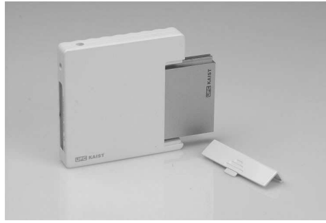
(b) Appearance of Zigbee Enabled Tiny Terminal with Case
