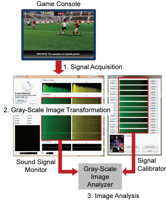
Fig. 3. The event detector module of PokerFace.
