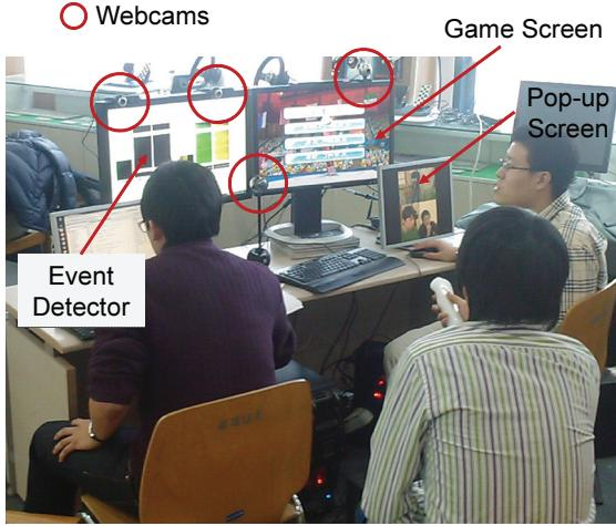
Fig. 4. A prototype implementation of PokerFace
