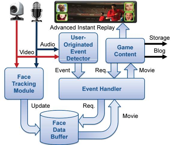
Fig. 2. The architecture of the PokerFace system.
